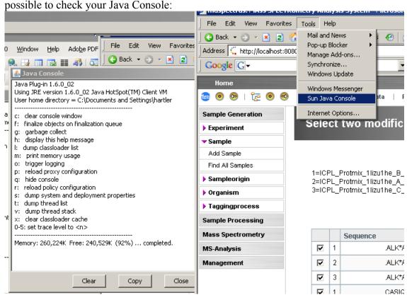
When you click in the Java Console on "m" you can check the memory used. The option –Xms is the permanently reserved memory and the –Xmx is the maximum memory that could be used if needed. When you start the Java3D viewer (clicking on the radio button Java 3D) and you get java.lang.OutOfMemory you have to less memory to run the 3D applet.
