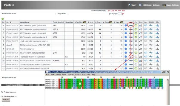
The procedure to display the alignment is similar to 7.2. First the "Load" button has to be clicked to start the alignment. On clicking the Java icon Jalview Alignment editor will be started to show the results.
